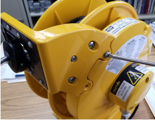
1. Completely remove the (2) inner screws.
