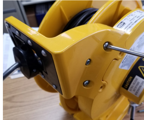
2. Just loosen the (2) outer screws, keeping the clamp plate attached to the roller guide.
