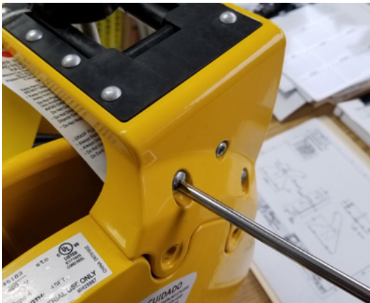
3. Remove and rotate roller guide and move to alternate location on the vertical frame for a vertical up position. (This position would be used if you are hanging your reel from the ceiling, for a lifting application)
