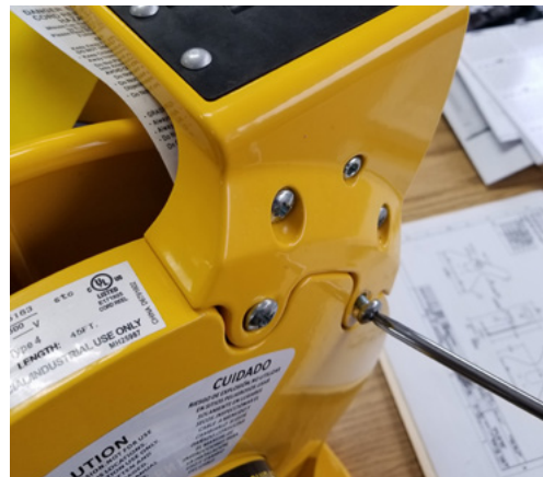
5. Re-assemble the (2) inner screws, and tighten as required.
